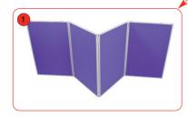
Take the 1st set of panels (with connecting clips) and open out until the above shape is achieved and stable. (ensure the connecting clips are at the top of the panels.
